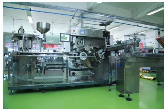
*The machine can now produce up to 450 blisters per minute thus making production much faster. Currently the PG Express machine is installed at a leading pharmaceutical manufacturer in India and running successfully.*
